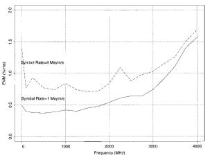
RF EVM performance versus frequency (root Nyquist filter, a = 0.25, ALC = off, modulation =  $\pi$ /4DQPSK)
