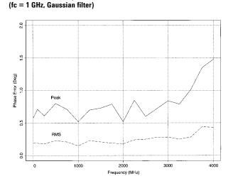
Phase error versus frequency (Gaussian filter, BbT = 0.5, symbol rate = 1Msys/s)
