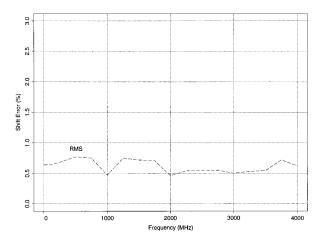
Shift error versus frequency (Gaussian filter, BbT = 0.5, modulation index = 0.5, symbol rate = 1Msys/s)
